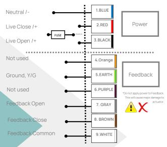
For Series 80-400, remove wiring box via 4 x screws. This will expose the wiring terminal. Simply match the colours and codes you see against the above. Then re fit the wiring box and ensure seal is in place. Standard Modulating including Failsafe and Hi-Speed Wiring: Series 80-110-200-400
