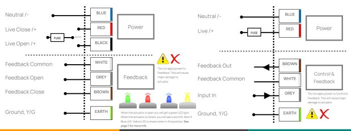
Standard On Off, Failsafe and Hi-Speed Open/Close Wiring: Series 80-110-200-400.
