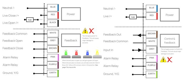
Standard On Off, Failsafe and Hi-Speed Open/Close Wiring: Series 80-110-200-400 with alarm
